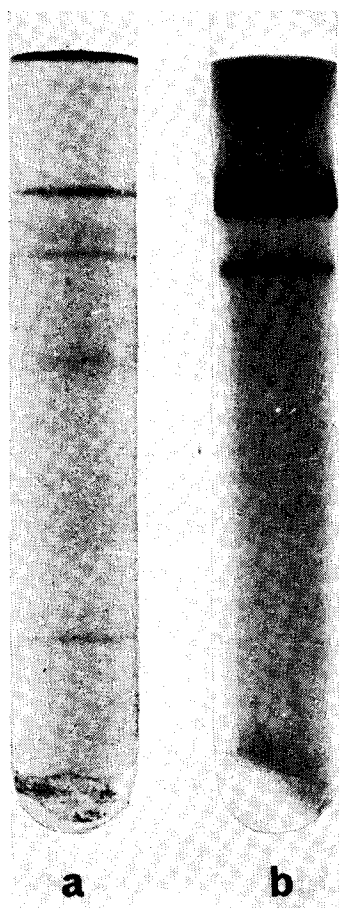
Fig. 3. Polyacrylamide electrophoresis of the soluble ATPase from E. coli . Aliquots (30–40 \mu g protein) of the soluble fraction after extracting the membranes with 3 mM EDTA–50 mM \text{NH}_4\text{HCO}_3 , pH 9.0, were electrophoresed as indicated under Materials and Methods. Migration was towards the anode (bottom of the gels). Gel a shows protein staining, Gel b illustrates the ATPase stain.
